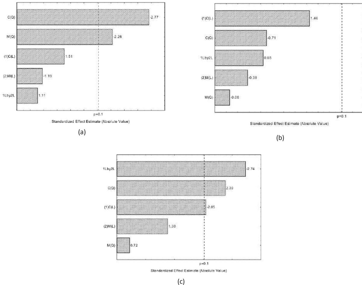
**Figure 2 Pareto chart showing the effects of linear, quadratic and interaction terms of independent variables on top ethanol concentration (a), bottom ethanol concentration (b) and recovery efficiency (c)**
