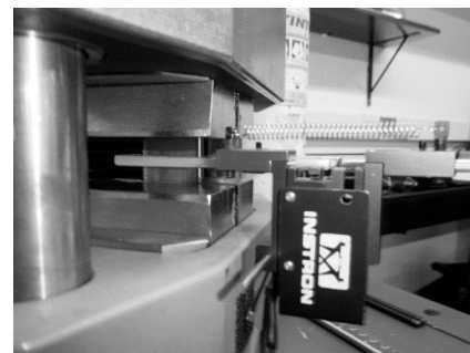
Figure 1 Extensometer with extensions for transverse strain measures
