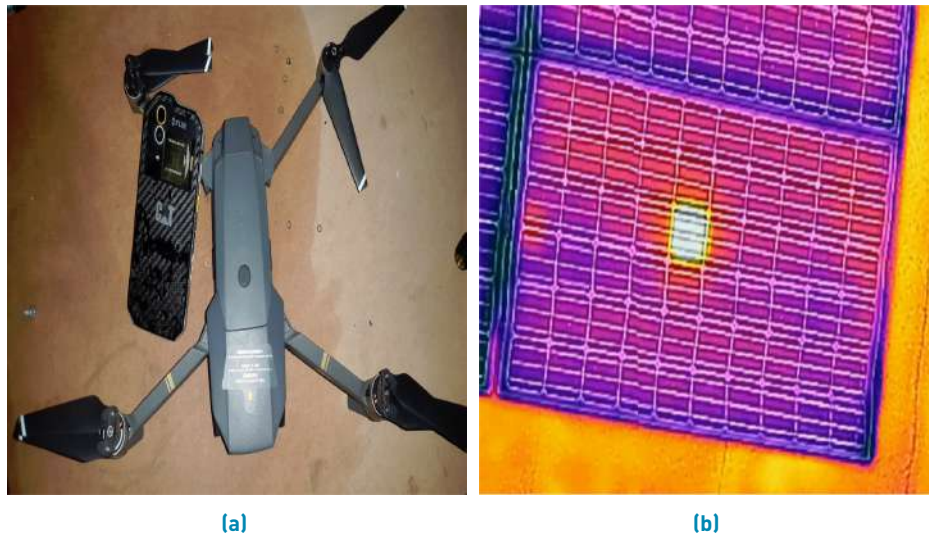
Figure 16 Solar panel thermography with drone (a) Cat s60 thermal camera and DJI Mavic Pro drone (b) captured image
