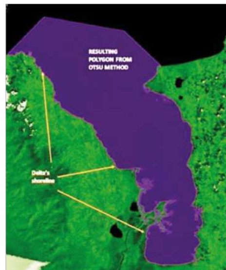
Figure 3 Polygon obtained after applied Otsu method, one of its sides is the shoreline of the delta
