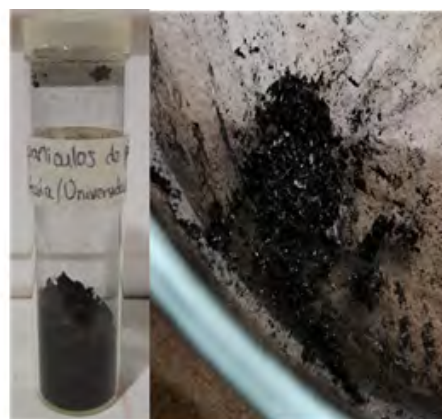
Figure 2 Silver nanoparticles synthesized using Musa paradisiaca extract as a salt reducing agent AgNO_3
