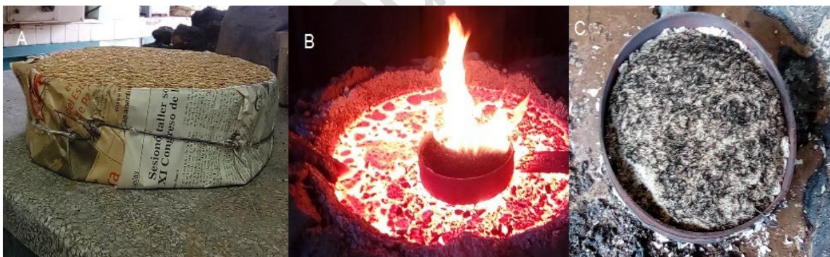
Figure 1 A, B, and C: Ring with the RH sample prepared to be placed on the newly poured steel, combustion of the RH sample on the AISI 1045 steel, resulting in RHA from the combustion.
