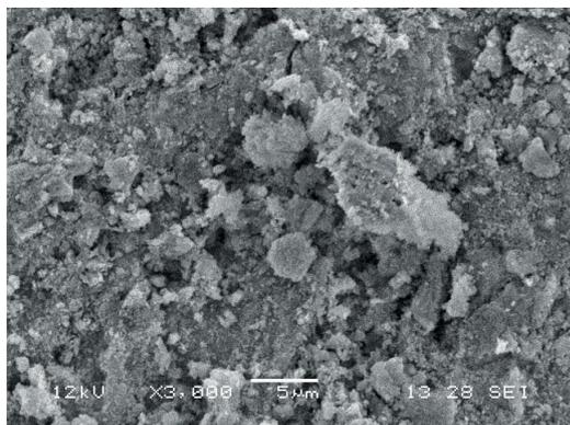
**Figure 9** SEM surface morphology of the ZnO sample, obtained by PEO with an electrical potential of 550 V. The behavior of the surface modification was similar using the other voltages
