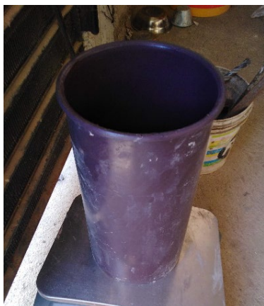
Figure 2 Mold for preparation of cylindrical specimens
