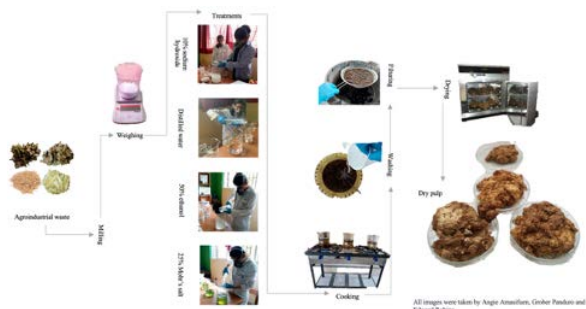
Figure 3 Delignification process of the AIW evaluated
