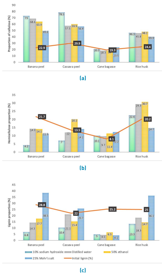
Figure 4 Final cellulose (a), hemicellulose (b), and lignin (c) contents for each waste after treatment
