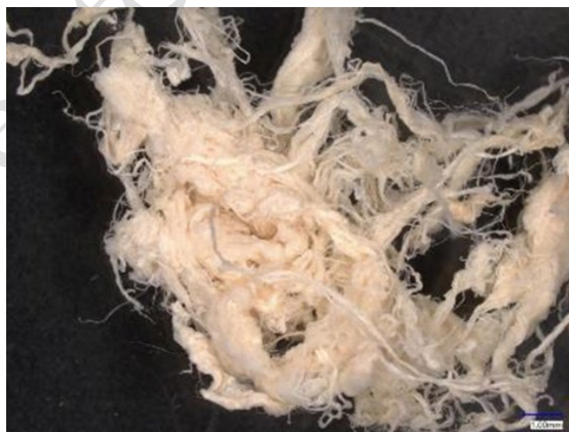
Figure 2 Sodium alginate fibers.
