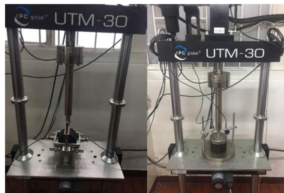
Figure 3 UTM for Resilient modulus (left) and permanent deformation tests (right)
