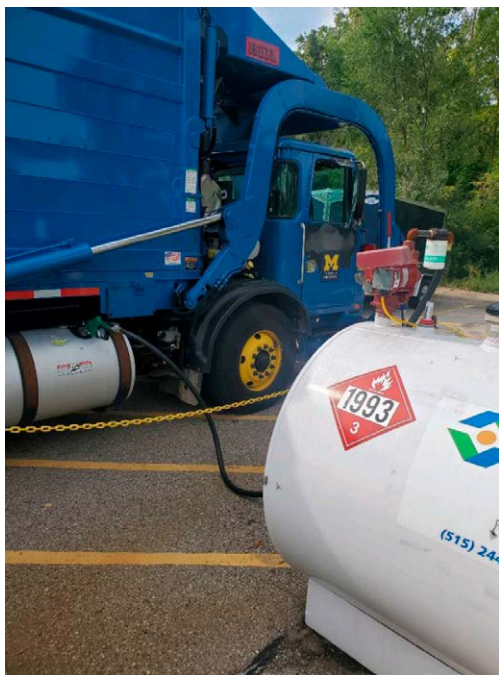
Figure 2 Test vehicle and refueling tank for 100% renewable fuel demonstration (R50B50) in a campus refuse truck, which show fuel economy parity despite the lower volumetric energy density of the renewable fuel. (photo credit: P. Chapman)
