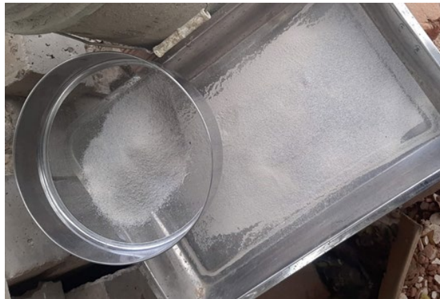
Figure 1 Glass crushing process and final sample in retained powder 0.075 mm.
