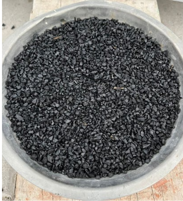
Figure 2 Texture of treated granulated rubber.
