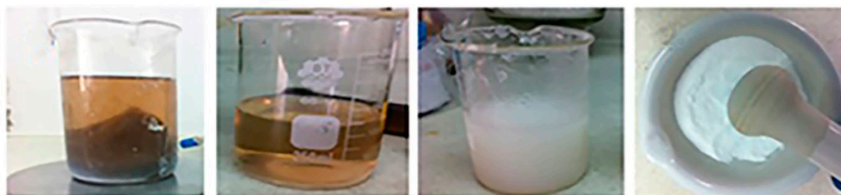
Figure 1. Products of the different steps of the amorphous silica extraction: (a) digestion of CCA in 2.5 M NaOH, (b) filtration of \text{Na}_2\text{SO}_3 , (c) silica gel, (d) amorphous silica.
