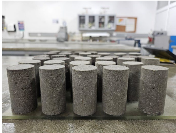
Figure 2. Alkali-Activated Hybrid Cement from Mining Tailings and OPC.
