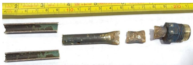
Figure 2. Siphon tube with fitting fractured during the disassembly.
