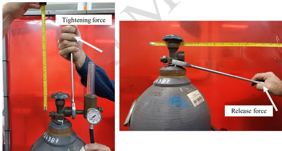
Figure 4. Cases for the analysis a) Normal operation. b) Valve disassembly.
