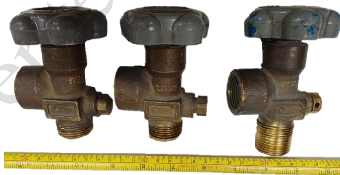
Figure 1. From left to right: Valve 1 and 2 (Failed), Valve 3 (without failure).
