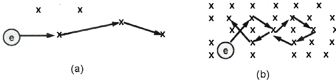
Figure 3. Illustration of two types of situations of weak electrical field of ionic nature for quasiperiodic structure (a) small dispersion center in the net and (b) concentrated dispersion center in the net.
