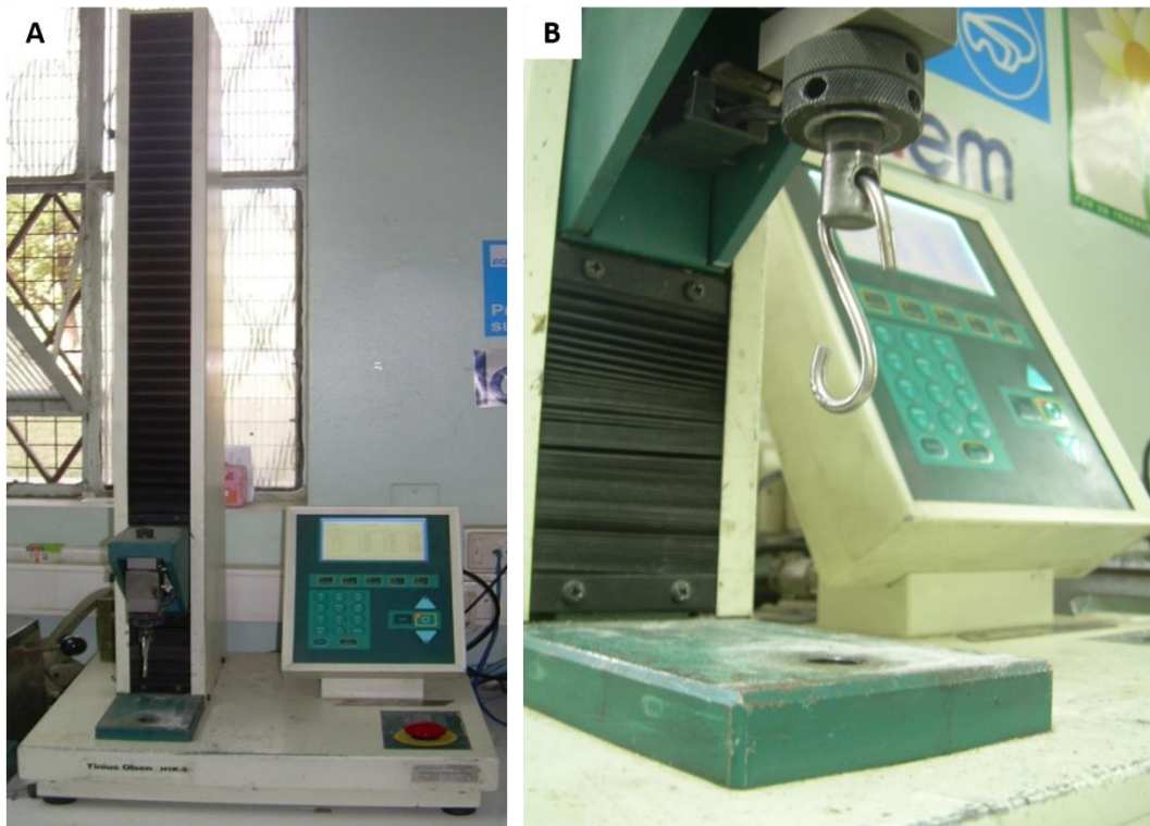
Figure 5. A and B. Device used for tensile testing (Tinius Olsen H5K-S)
