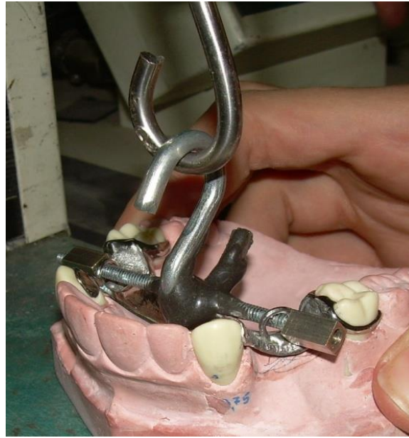
Figure 6. Traction device installed on metal bases to run the test
