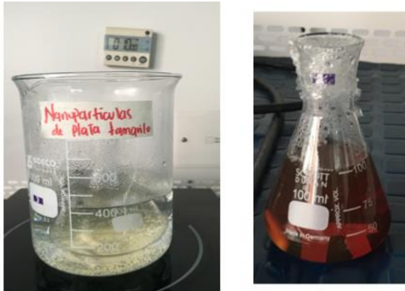
Figure 1. Synthesis of solid silver nanoparticles and suspension by obtaining tree tomato and guava extracts. The color change of the solution over time indicates the presence of nanoparticles in it.
