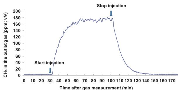
**Figure 4.** An example of methane recovery tests. The standard gas was released starting at 30 min and continued until 100 min. The basal concentration of CH<sub>4</sub> was calculated based on the data during the first 30 min. Recovery rate (%) was calculated as the ratio of the recovered amount of CH<sub>4</sub> gas to injected amount of CH<sub>4</sub>.
