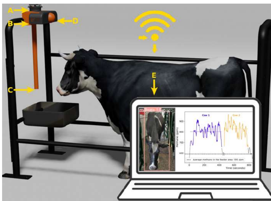
Figure 1. Schematic representation of the integrated methane measurement and identification system installed in a milking stall: A) Air pump, B) Protection box housing electronics, C) Air sampler, D) Camera for cow identification, and E) Central laptop for receiving information via Wi-Fi from the device.
