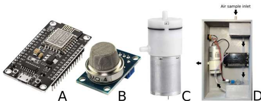
Figure 2. Components of the methane emissions recording device. ESP8266 Wi-Fi module (A), MQ-4 gas sensor (B), air pump (C), and plastic box containing the electronic and mechanical components (D). The arrows indicate the airflow direction.
