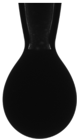
Figure 2. A droplet of CAG 0.25%. Goniometer ramé-hart instrument co. Model 290-U4 serial No. 200205
